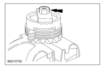
7. Select and insert the thickest feeler gauge blade that will enter between the tool and the differential clutch pack. The reading will be the thickness of the new clutch shim.
