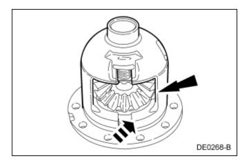
12. Using a soft-faced hammer, install the differential clutch spring.
