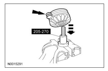
4. Position the Differential Clutch Gauge hand-tight on top of the differential clutch pack.
