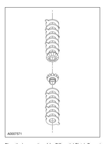
3. Place the base portion of the Differential Clutch Gauge in a vise. Install the differential side gear and differential clutch pack (without the shim) on the tool.
