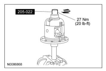
19. Install the differential carrier. For additional information, refer to <u>Differential Carrier</u> in this section.
