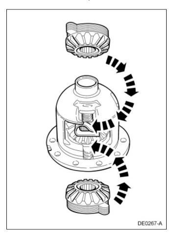
11. Install the 2 differential pinion gear and differential pinion thrust washer assemblies in the differential case.
