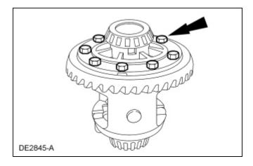
3. **NOTE:** Care should be taken not to damage the differential ring gear bolt hole threads.
