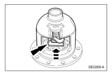
13. Install the differential pinion shaft and install a new bolt finger-tight without tightening into the loctite covered area of the bolt.
