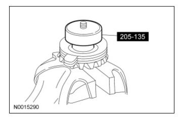
5. Install the Differential Clutch Gauge over the disc and differential clutch pack.
