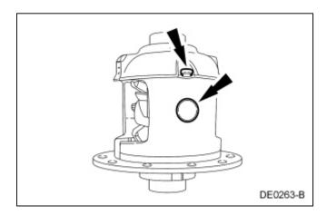
7. **NOTE:** Due to the spring tension, care must be used when removing the differential clutch spring.
