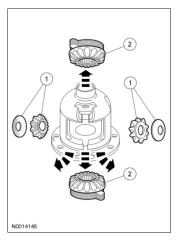
9. **NOTE:** Keep the differential clutch packs in order. Do not mix the differential clutch packs. The differential clutch packs must be reassembled in the same sequence.
